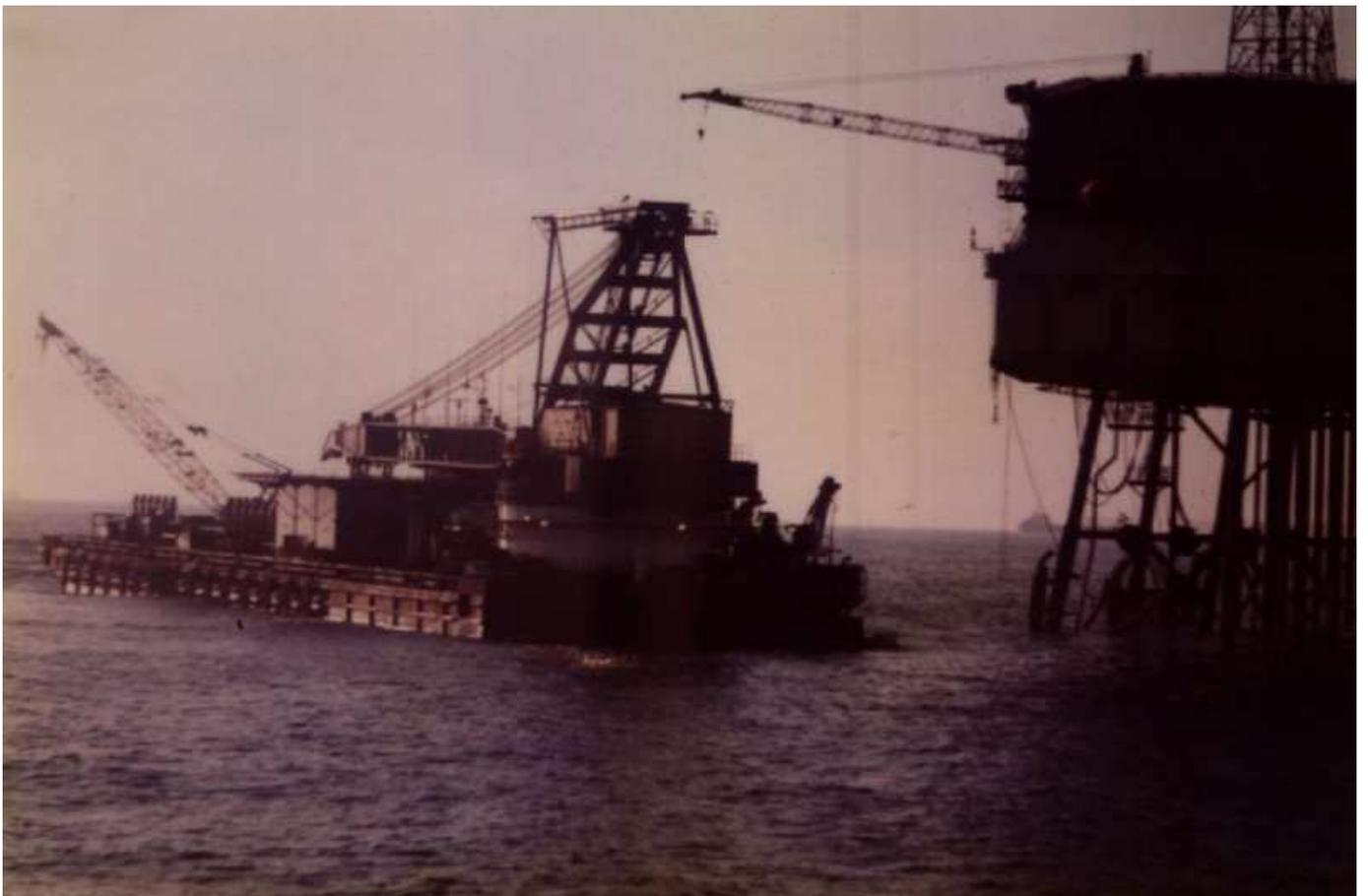
This is a Barge, Brown & Root Pipe Lay Barge "BAR 297".
