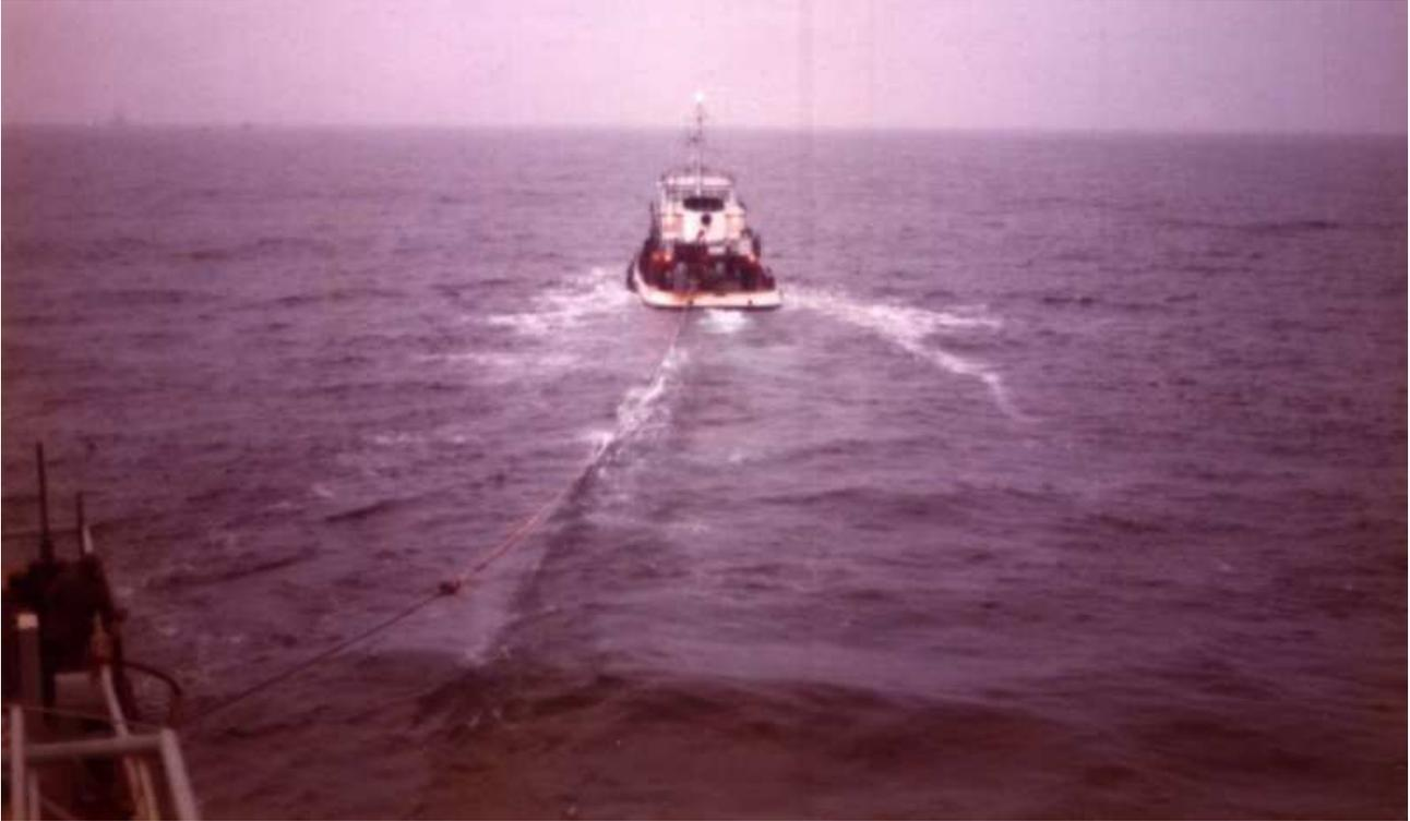
The barge has no engines, it is towed by a Tug Boat at the end of a long cable.
