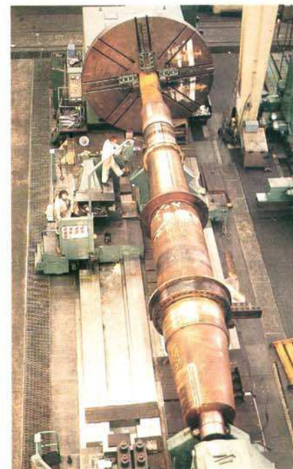
Machining a damaged rudder stock of a VLCC at the WF-RDM General Engineering Works.
